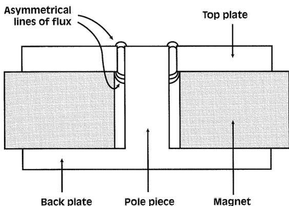
The uneven lines shown in Figure 1. create an asymmetrical magnetic flux field which results in higher distortion. Both the Infinity/Watkins dual voice coil woofer and midbass coupler utilize an extended pole piece which creates symmetrical lines of flux in the magnetic gap as shown in Figure 2. This significantly lowers distortion.
