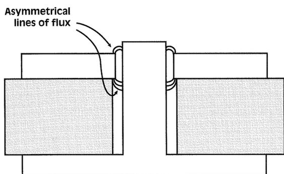
The voice coil operates in the magnetic field generated between the top plate and pole piece, and a symmetrical flux field translates the voice coil's current into an up and down motion that is a close replica of the speaker's input signal. Obviously, closer adherence to the original signal results in less audible distortion which is readily identifiable in a high quality, totally transparent speaker. In addition to the symmetrical magnetic flux field design,
