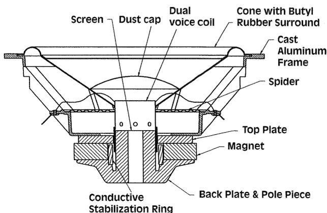
The Omega Series woofer is the best performing Watkins-woofer Infinity has ever made. Without being able to rely on the very costly Servo Feed-back systems found in more expensive Infinity loudspeakers, the Omega woofer, takes several novel approaches to Low-Distortion Low-Frequency Response.
