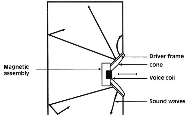
2. Sound pressure waves within the enclosure are formed by the moving cone as it responds to input signals. These pressure waves can generally be damped by using dacron or a similar material inside the enclosure. The choice of the proper material and density of the material is of critical importance for the proper absorption of unwanted energy. Refer to diagram 2.
